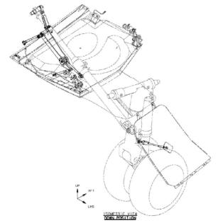
Figure 1: Retraction actuator acting as side stray
